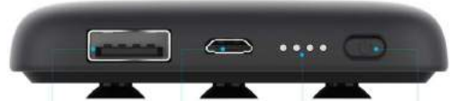
Spare USB Port Output 2.1A (Max) Micro USB Input 2A, Output 2.1A (Max) (for charge and discharge) Capacity Display 25% 50% 75% 100% Button Press to show capacity level
